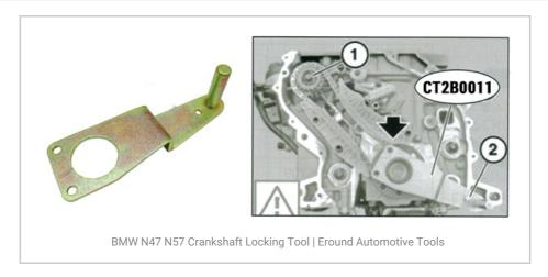
The crankshaft must be blocked in order to release central bolt (1) of the high pressure pump. Position special tool CT2B0011 with screw (2) at the crankcase. Release central bolt (1) of high pressure pump. Important! Release central bolt only, do not remove.
